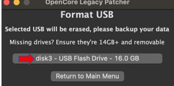
The installer will create macOS installer Ventura on USB stick which will be used to boot later
