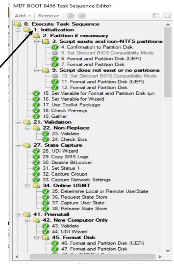
With this extension it will be easy to troubleshoot error during build because smsts.log will contain the step number where the build failed and the reason.
